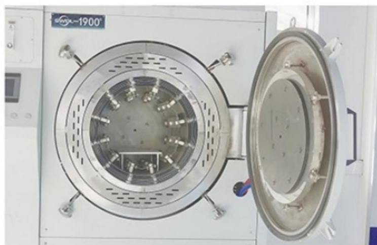
高温真空烧结炉—加热室 High-temperature vacuum sintering furnace
